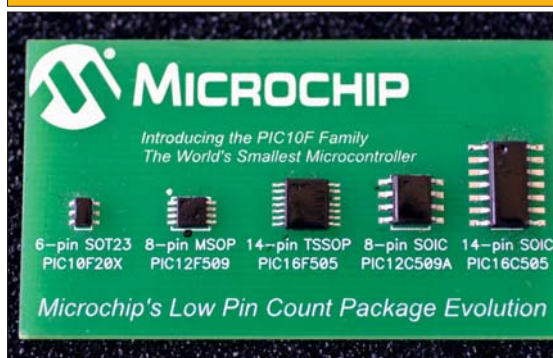
Figure 1. Yep, the PIC10F206 is a tiny bugger, but it's still big enough to allow you to hang some wire-wrap wire off of its pins or solder it onto a set of SOT-23 copper pads.
